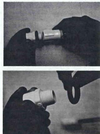
Unscrew the male adapter from the female adapter then remove the o-ring from the male adapter.
