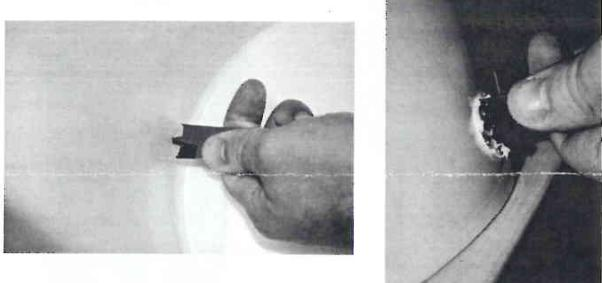
POWER DRILL NOT REQUIRED. THIS CAN BE DONE BY HAND. Drill a 22 mm (13/16") hole in the side of the pail by twisting the hole cutter (B) about 38 mm (1.5") from the bottom of the bucket. This height will prevent sediment from entering the filter.
